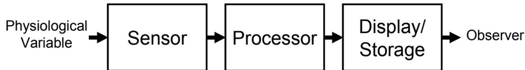
Figure 1.1. Block diagram of a general instrumentation system.
